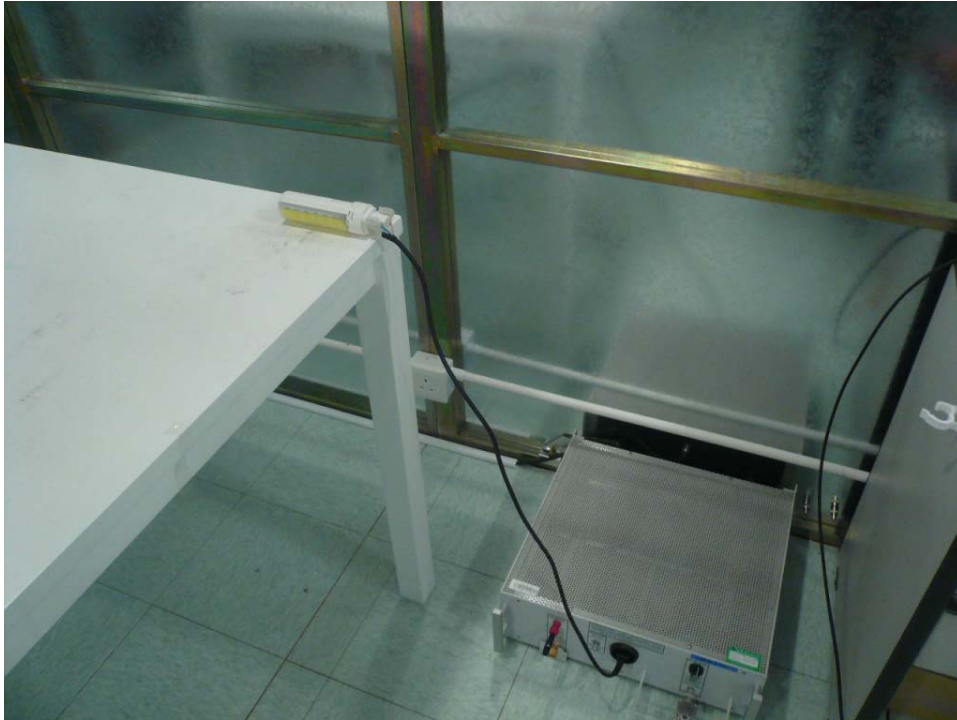
Figure 3 Conducted emission test setup
